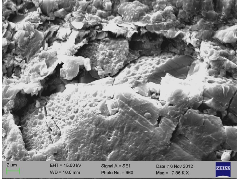
Figure 3.34 St-1- Heidelberg field/4,916-5,581 ft SEM image shows cavity in calcite embedded in clay matrix. Cavity exhibits karst-like structure more like pock marks (post-carbon dioxide).
