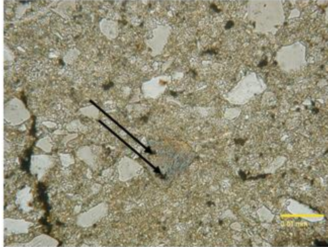
Figure 3.15 Ssm-3- Sandstone (Heidelberg field)- 15231-15246 ft Photomicrograph shows voids in grain, possibly dissolution features and also note fracture on left corner. Arrows point to dissolved microcline (post-carbon dioxide).
